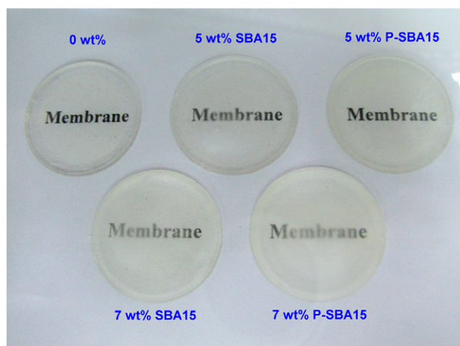
Fig. 2. Photographs of resulting PMMA/IL composite membranes containing various amounts of mesoporous silica fillers.
